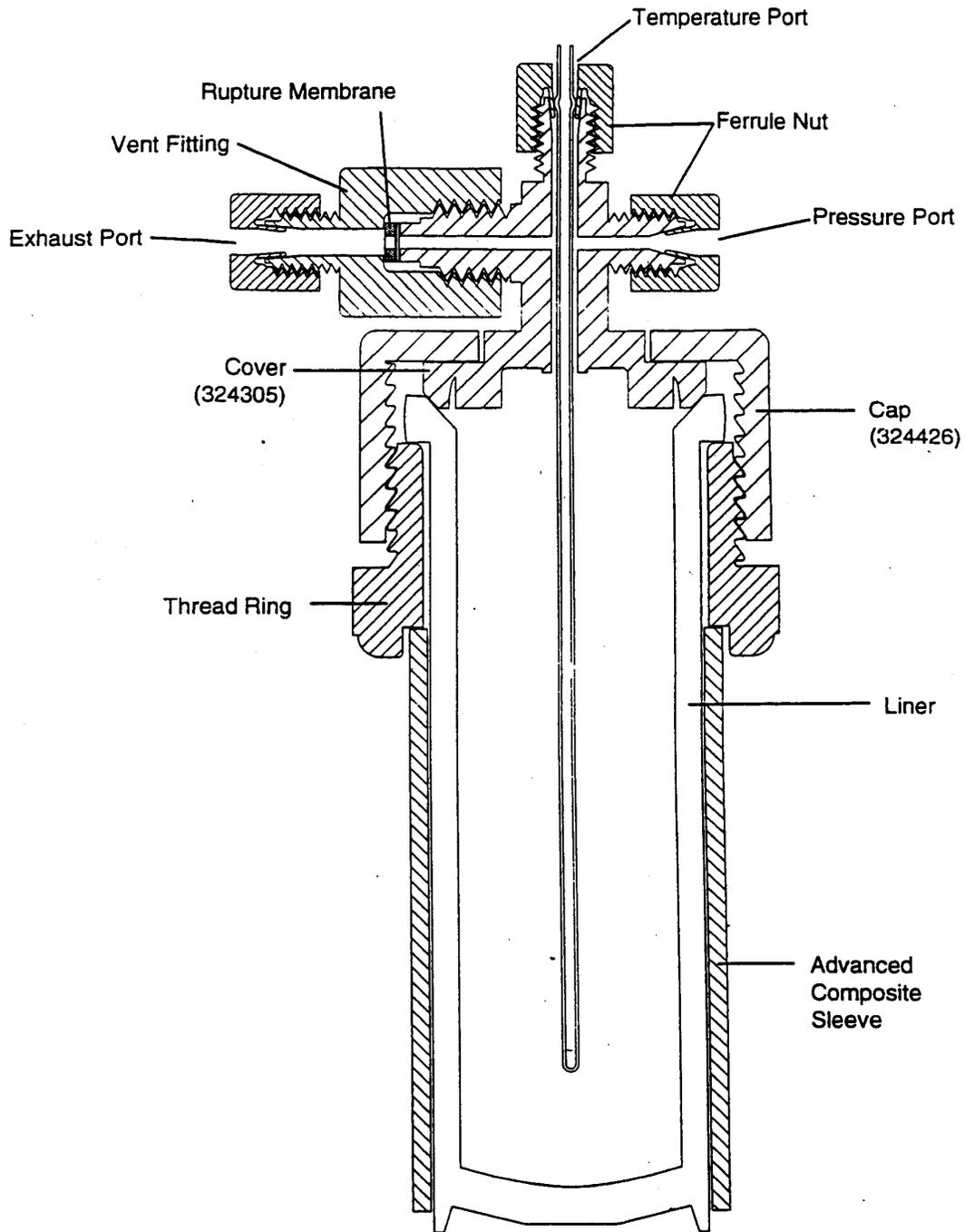
Figure 2. Advanced composite vessel for pressure and temperature control.
