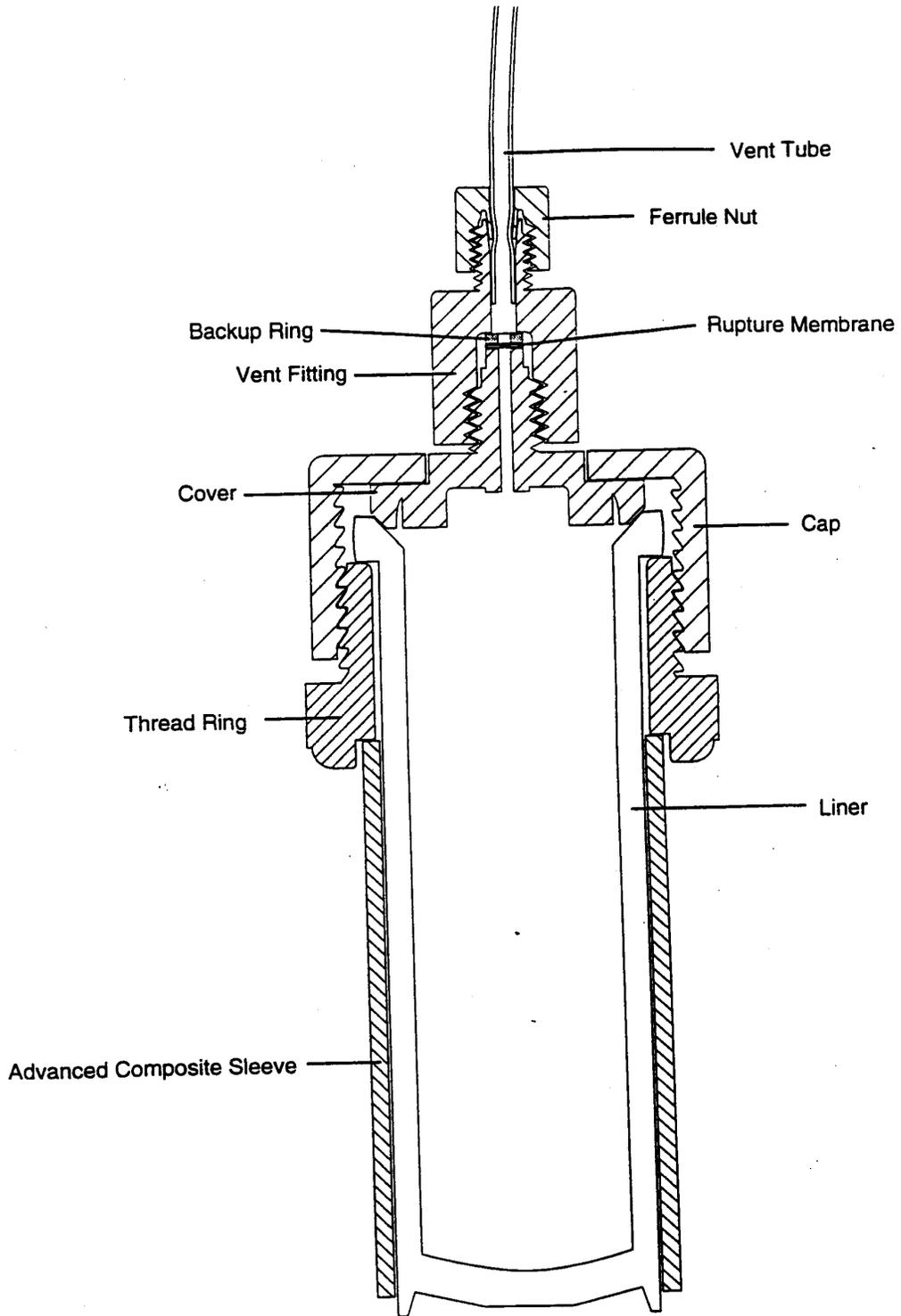
Figure 1. Standard advanced composite vessel (cross section).
