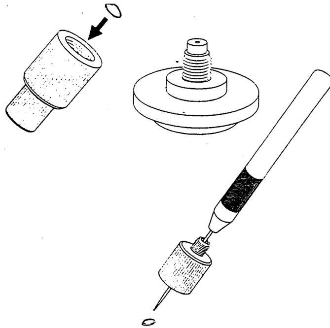
**Figure 3.** Installation and removal of rupture membrane.
